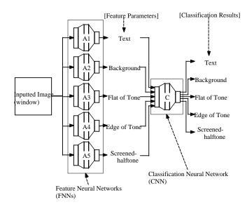
Figure 3: NN structure for the classification (CNN).
