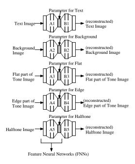
Figure 2: NN structure for the feature extraction (FNNs).
