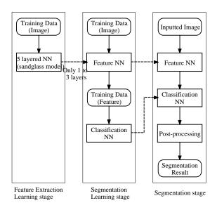
Figure 1: Flow diagram of segmentation using NN.
